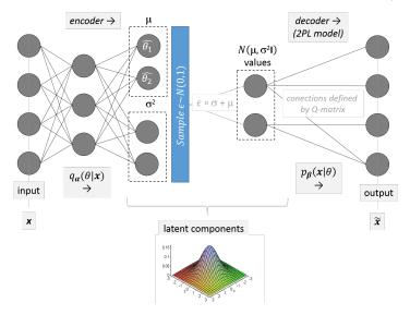
Proposed modification: no hidden layer in the decoder (2PL) and output layer not dense (non-negative weights).
